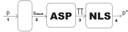
Fig. 2. Follower System: applies the Approximation Strategy Property (ASP) and constructs a permutation \pi that follows the corresponding strategy s^{id} (that would get the exact probability of occupation of the input).
